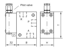
Externally pressure controlled relief valve type AE, size 4, manifold mount-
