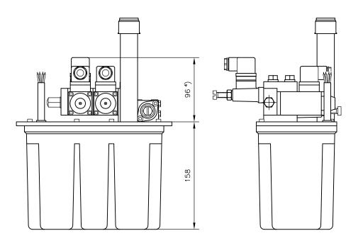
Mass (weight) = 6.1 kg (basic pump without oil filling)
