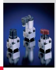
These valves may be directly installed in pipe systems, when equipped with subplates enabling pipe connection. Many optional functions can be incorporated in these sub-plates e.g. pressure limiting valve or restrictor check valve for widen the field of application for this valve type. Valve banks of these valves are also available featuring several valves connected in parallel (see type VB).
