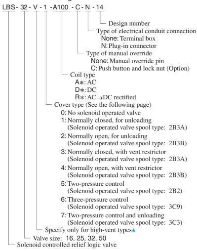
★ Use high-vent pressure types if the shifting time from unloading to on-loading is reduced.
